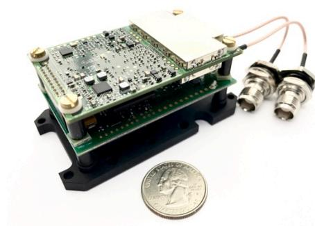
The Inertial Labs **INS-D/DL-OEM** utilizes advanced dual antenna GNSS receiver, 3-axes each of calibrated in full operational temperature range Advanced MEMS Accelerometers and new generation of tactical grade MEMS Gyroscopes to provide accurate Position, Velocity, Heading, Pitch and Roll of the device under measure.
